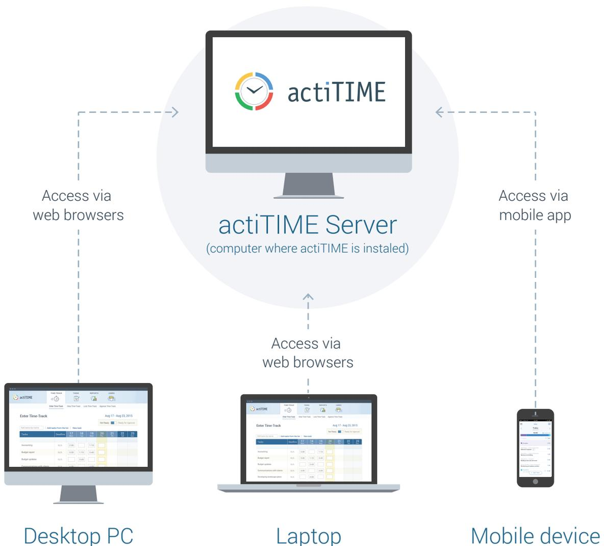
There's no need to install actiTIME on each computer. Just install it on one machine and make sure it is accessible from outside:
